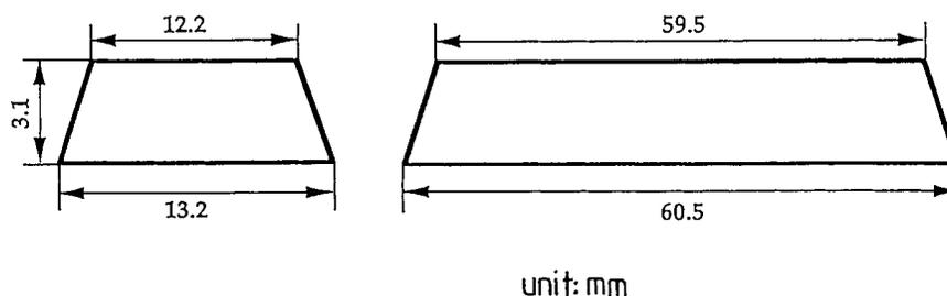
Figure 3 Bending specimen geometry.
