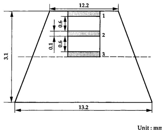
**Figure 2** Schematic representation of injection molded PPS/LCP sample; (1) skin layer, (2) boundary, and (3) core layer.
