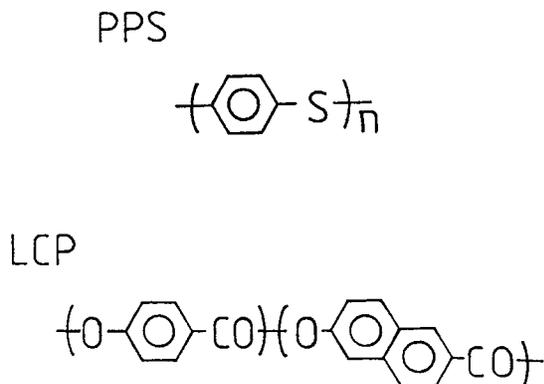
**Figure 1** Structures of PPS and LCP.
